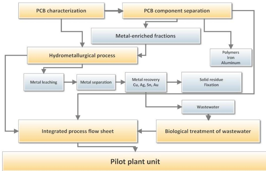
Figure 2. Schematic diagram of the concept of PCBHYDRO Project.
